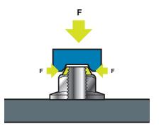
This elasticity makes it possible to screw Nedlock several times without a complete loss of clamping torque and seizing issues.
