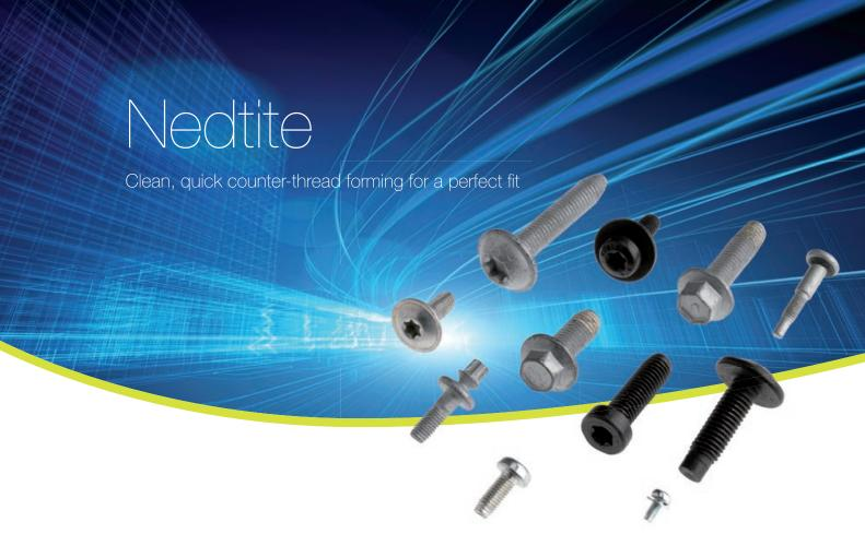
Nedtite screws are a cost-effective solution for direct mounting in light metals and different types of steel. The key innovation here is the trilobular geometry of the shaft. This allows the screws to form their own counter thread in a drilled, cast or deep drawn hole which remains entirely free of metal chippings or dirt. No preparation is required. A nut thread, in which the screw is assembled, is no longer necessary.
