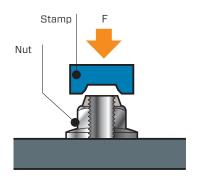
Nedlock's segmentation is 'bent' slightly inwards which results in a radial tension in the segment region, with largely elastic behaviour.
