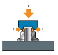
This elasticity makes it possible to screw Nedlock several times without a complete loss of clamping torque and seizing issues.
