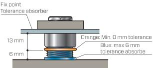
The outer part, with its welding humps, takes care of the initial attachment. The smallest metal part with M16 thread makes an axial rotation and bridges part of the distance. The smaller M8 thread ensures solid fixing.
