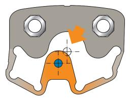
Flexible plate bars allow durable deforming for precise adjustments in final production phase.
