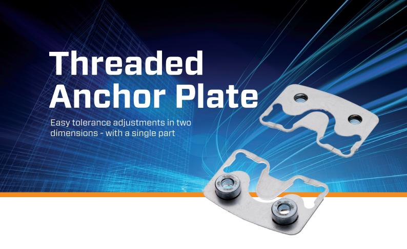
Nedschroef's anchor plate combines a robust and durable fixation area with the possibility for tolerance adjustment - in one single part. This is done by deforming the flexible bars in the plate. Our unique solution is applied in the automotive industry for the adjustment of door locks, at the end of the assembly process, allowing the customer to make precise adjustments in the final phase of production.
