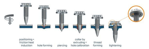
By piercing its own hole, making a channel and forming its own thread, Nedtite ES creates a low hole and thread forming torque and a very high overload torque for fixing.
