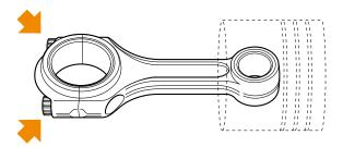
The new generation of Nedschroef Ultra Fasteners enables a more compact design of the connecting rod, and therefore also a more compact design of the crankshaft. This saves weight and space of all components in the joint and allows complete engine downsizing.
