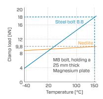
Counterparts are made of lightweight metals with lower tensile strength, such as aluminium or magnesium. With aluminium fasteners, the threaded hole doesn't need to be as deep as with steel fasteners. This reduces drilling- and thread cutting time. The counterpart can be designed to be lighter, to save on cost and weight.
