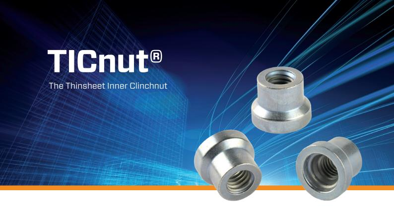
The new TICnut® satisfies today's demand for connecting elements that are compatible with ever-thinner sheets, sandwich panels and an increasingly diverse range of materials. The TICnut® can be used as a fixing element for multilayer sheet metals, when thickness is between 0.1 and 1.2 mm. A securely fixed washer can be combined with a rotatable nut (combi-element). With a special adjustment, the TICnut® can also be used as a tolerance absorber.
