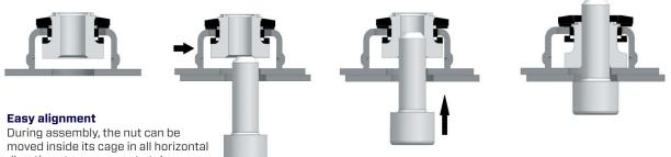
directions to compensate tolerances of up to 3 mm, enabling it to adapt its position to a misaligned component.
